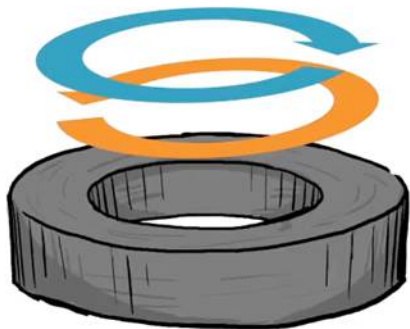
Persistent current in a superconducting circuit
